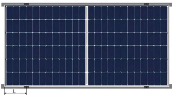
Clamps mounting Mounting rails cross the long frame(Method 5 )
